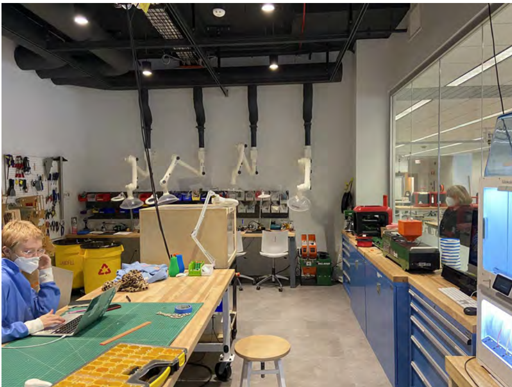
Figure 5.58 - Lasercutting (dirty maker), enclosed with glass to control dust. Note snorkels on the back wall for exhaust.
