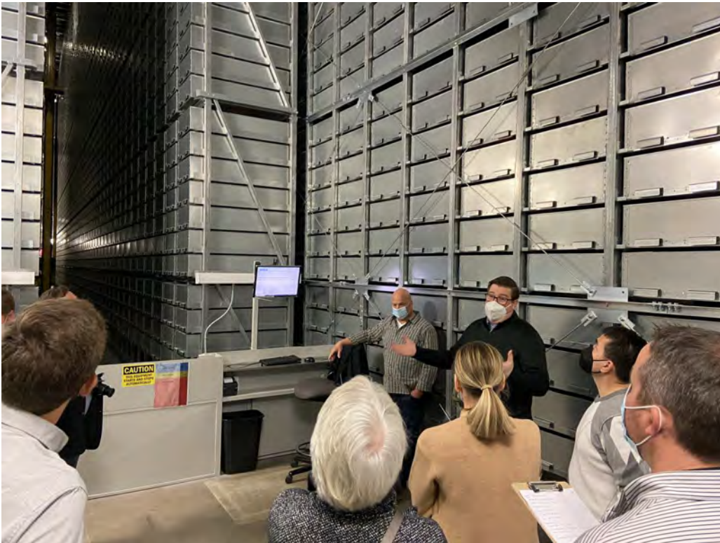
Figure 5.68 - Underground automatic storage and retrieval system (ASRS)
