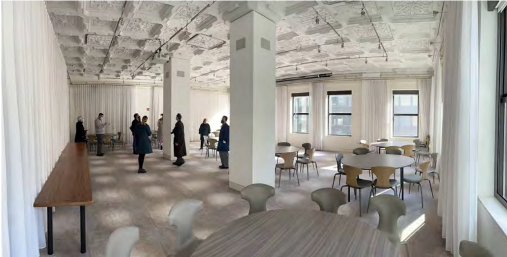
Figure 5.79 - Ballroom. Use of curtains at perimeter helps to hide storage and provide acoustic help.
